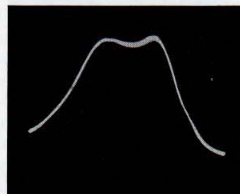
Fig. 76. Total response of first and second I.F. transformers and input of discriminator. Input signal applied to tap on oscillator coil L_{13} . Oscilloscope connected to point P on discriminator.
