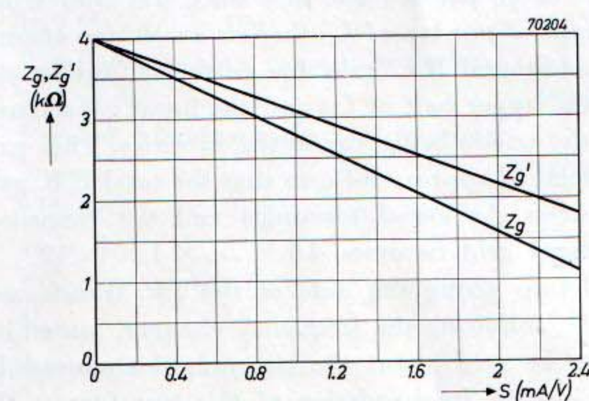
Fig. 66. Impedance of the grid circuit of the H.F. tube without feedback ( Z_g ) and with feedback ( Z'_g ) plotted against the mutual conductance for a frequency of 94 Mc/s (resonant frequency of input circuit).
