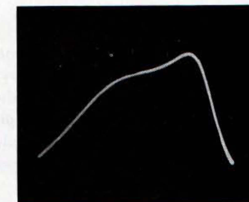
Fig. 72. Total response of second I.F. transformer and primary of discriminator. Input signal applied to control grid of heptode section of second ECH 81 tube. Oscillograph connected to point P on discriminator.
